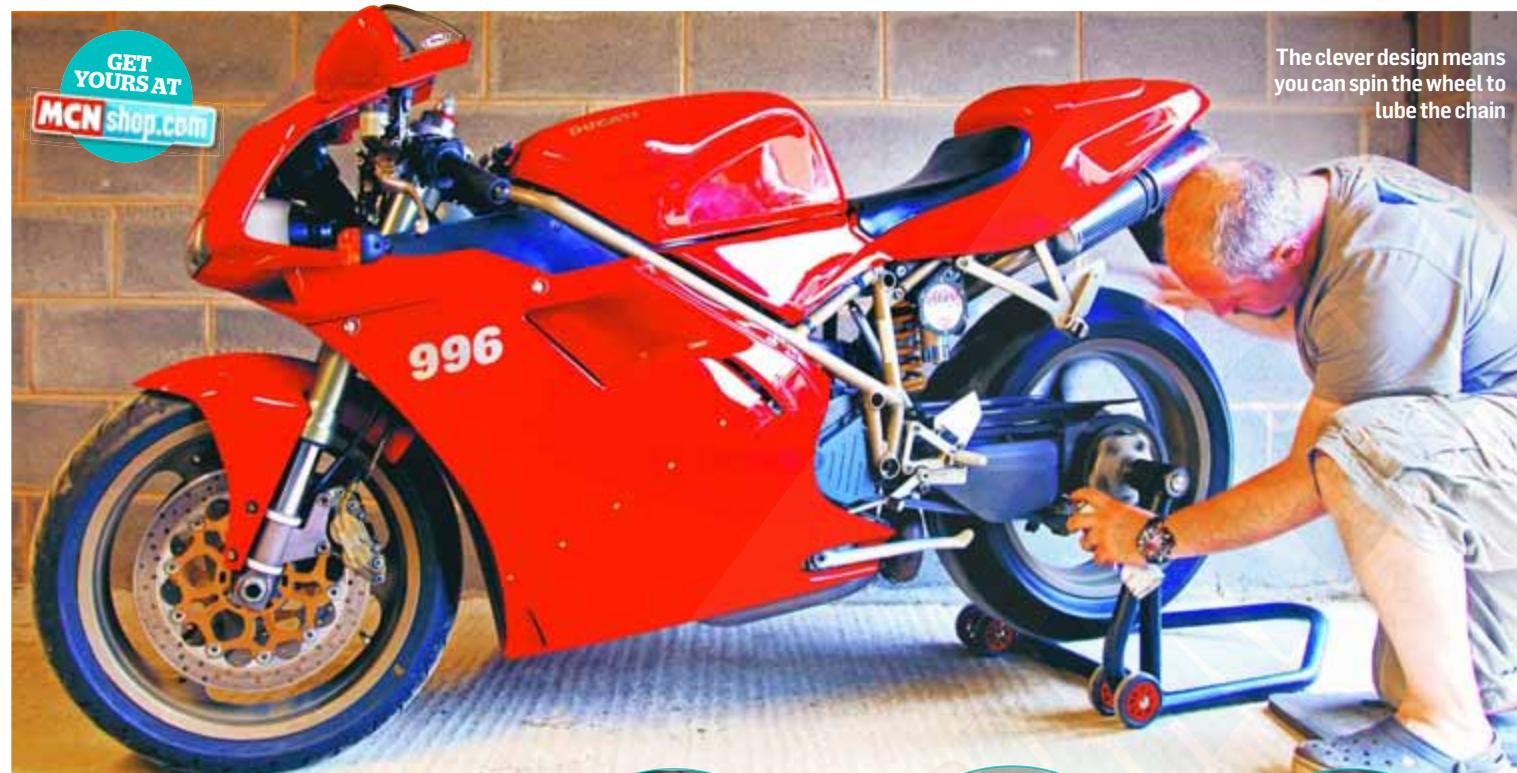
The clever design means you can spin the wheel to lube the chain
