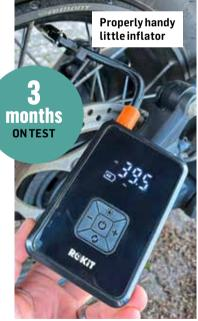
switches off automatically. It's even accurate against my proper gauge. It only measures 12.8x8x5.5cm, so easily fits in a rucksack or pannier without taking up much room.
