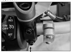
(Appropriate setup shown of the clutch lever housing when repositioned)
